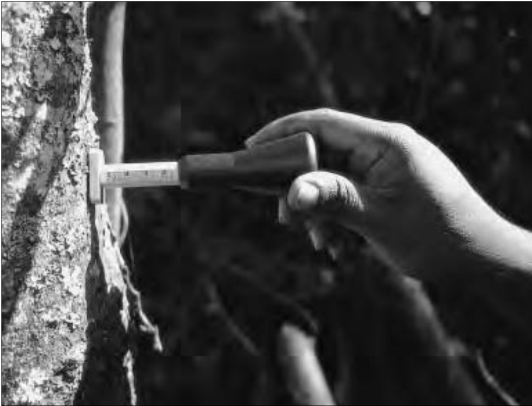
Figure 4.4 A Swedish bark gauge being used to measure the thickness of Prunus africana bark
